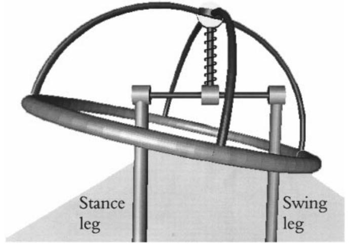
Fig. 10. The compensator body acts as an unactuated pendulum in the frontal plane, preventing the walker from tipping over sideways.
