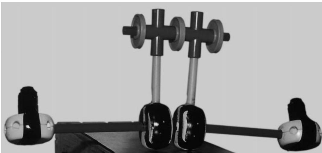
Fig. 2. Coleman's<sup>7</sup> prototype of a straight legged 3D walker, constructed with TinkerToys™.
