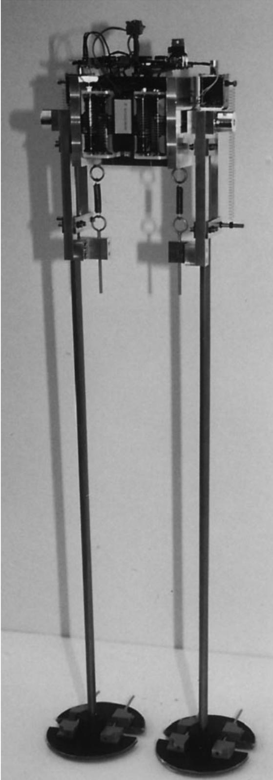
Fig. 3. Van der Linde's<sup>8</sup> powered straight legged 2D walker.
