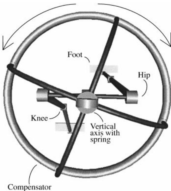
Fig. 9. Top view of our model. An oscillating compensator body counteracts the change in angular momentum from the swinging legs.
