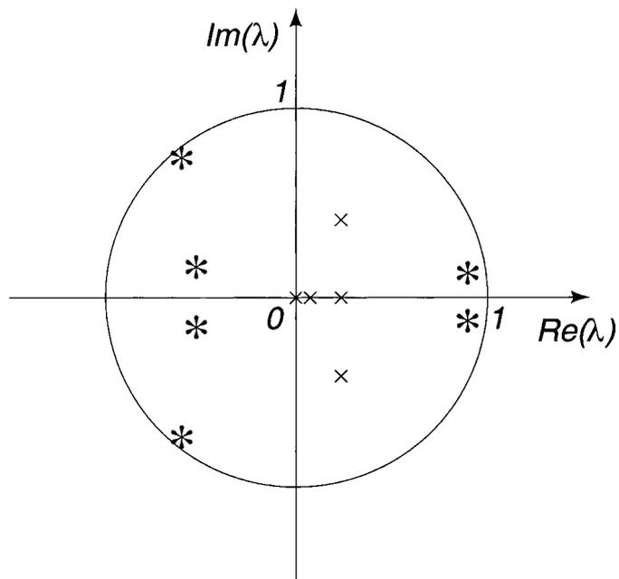
Fig. 13. Stability of the semi-3D model with a yaw compensator. The \* indicates the extra *eigenvalues* from the extension of the 2D version to the 3D model with a pelvic compensator body.
