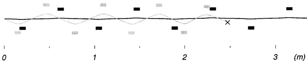
Fig. 12. Projection of the path of the center of mass on the floor. Without compensation (gray), the zigzag walking motion fails after eight steps. With a pelvic compensator (black) the robot walks straight and stably.
