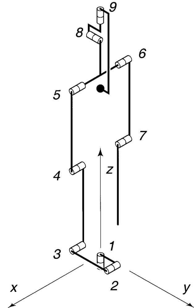
Fig. 6. Degrees of freedom of our 3D model. The massless swing foot doesn't influence the overall dynamics, and is therefore not displayed.
