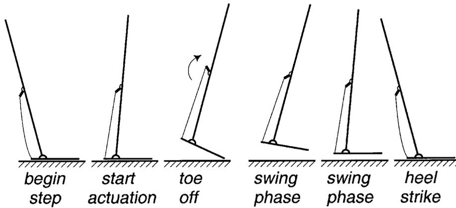
Fig. 8. Actuation scheme of ankle. During the first part of the stance phase, the ankle acts as a free joint. When the string becomes stretched, the actuator shortens the string, so that the walker rises on its toes. When the other foot hits the floor, the actuator releases the string. A small torsional spring in the ankle will keep the string stretched during the swing phase.
