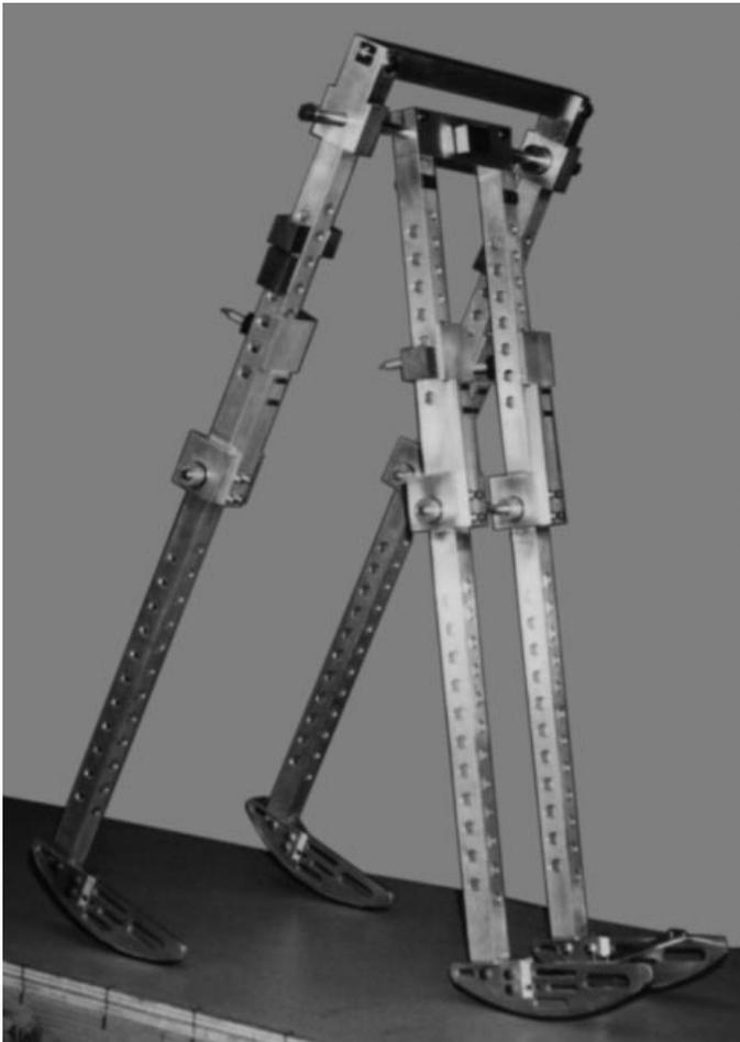
Fig. 1. Close copy of McGeer's prototype of a kneed 2D walker, by Garcia *et al.*<sup>4</sup>
