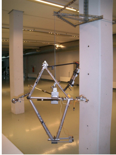
Figure 5: The rear frame clamped in the torsional pendulum.
