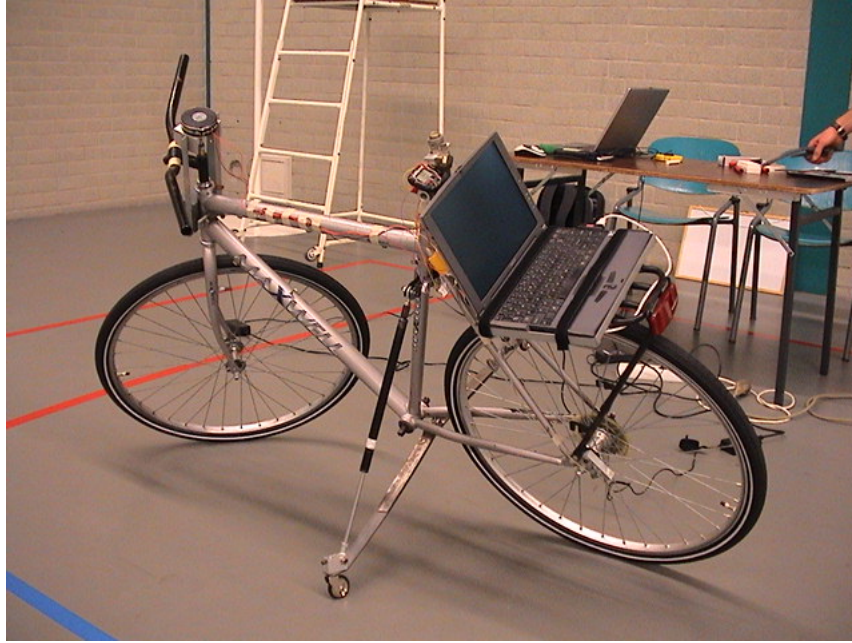
Figure 4: The instrumented bicycle with all the measurement equipment installed.
