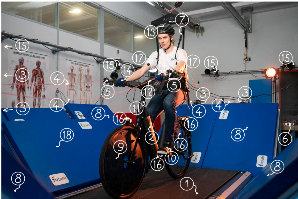
Fig. 1. Overview of the experimental setup, with: 1-treadmill, 2-bicycle, 3-pull force motor (4), 4-pull rope (4), 5-force sensor (4), 6-Speedgoat real-time controller, 7-intelligent harness, 8-soft padding (8), 9-disc wheel cover (2), 10-foot strap (2), 11-mechanical rotation limiter, 12-rear-brake handle, 13-helmet, 14-protective gloves (2), 15-motion capture camera (12), 16-IMU (4), 17-EMG measurement unit (4), 18-folding fence.
