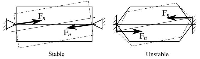
Figure 6. Grasping with pointed fingers (left) is stable, whereas with flat finger tips (right) is unstable.
