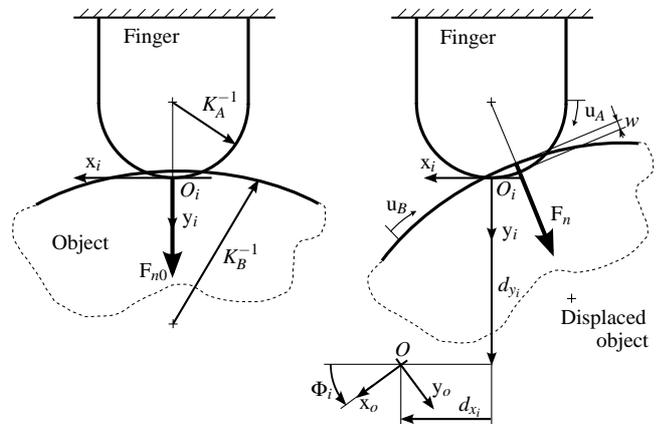
Figure 2. Local surface frame and orthogonal frame at a contact point, adapted from [1].
