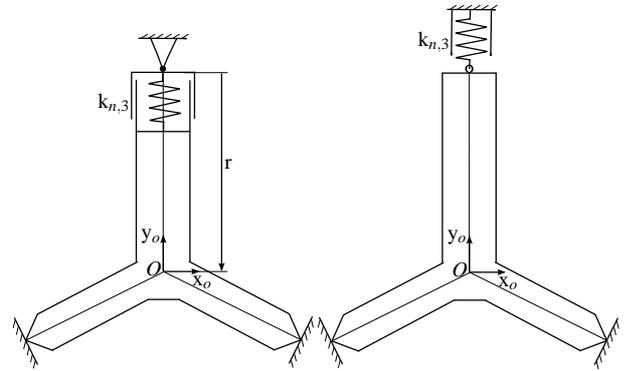
Figure 5. Grasp with finite stiffness at contact 3 in the object (left) and in the finger (right), respectively.
