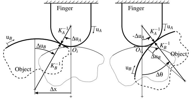
Figure 3. Relative motion of the object by slip (left) and roll (right).
