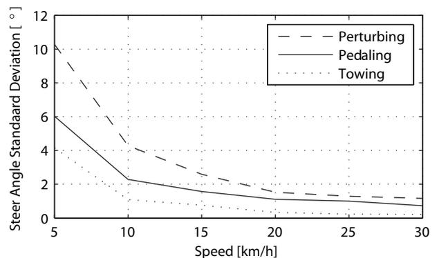
Figure 9. THE STANDARD DEVIATION OF THE STEER ANGLE FOR THE SIX DIFFERENT SPEEDS FOR THE THREE DIFFERENT EXPERIMENTS.
