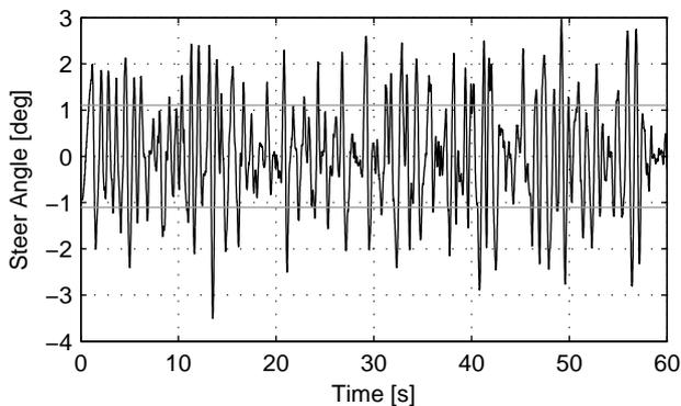
Figure 7. STEER ANGLE TIME HISTORY PLOT FOR 20 KM/H DURING NORMAL BICYCLING. THE STANDARD DEVIATION OF THE STEER ANGLE IS SHOWN IN GREY.
