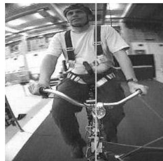
Figure 13. SCREEN-SHOT DIRECTLY AFTER A PERTURBATION (LATERAL FORCE APPLIED FROM THE RIDER'S RIGHT BY A ROPE AT THE SADDLE TUBE) AT 5 KM/H. VERTICAL GREY LINE INDICATES THE BICYCLE MIDPLANE. NOTE THE LATERAL RIGHT KNEE MOTION AND STEERING ACTION AND THE SMALL UPPER BODY LEAN ACTION.
