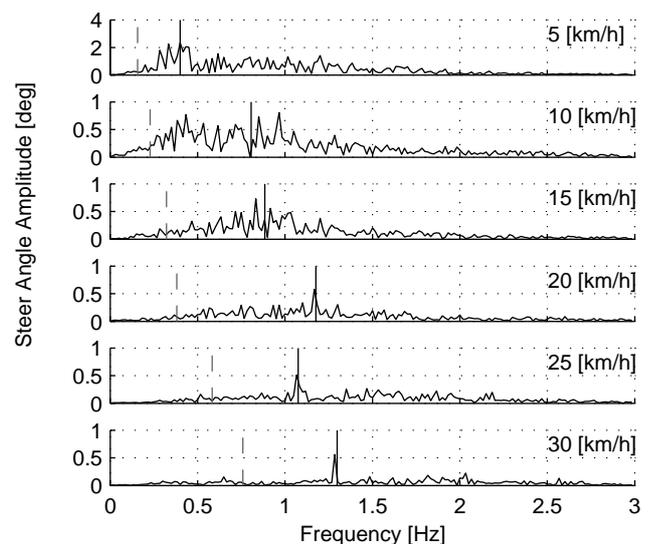
Figure 10. STEER ANGLE AMPLITUDE PLOT FOR THE SIX DIFFERENT SPEEDS FOR NORMAL PEDALING EXPERIMENT. SOLID VERTICAL LINE INDICATES THE PEDALING FREQUENCY. DASHED VERTICAL GREY LINE INDICATES THE BICYCLE & RIGID RIDER WEAVE EIGENFREQUENCY.
