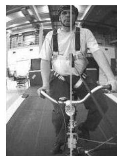
Figure 6. SCREEN-SHOT OF NORMAL PEDALING AT LOW SPEED (5 KM/H) SHOWING LARGE LATERAL (LEFT) KNEE MOTION AND (RIGHT) STEERING ACTION. THE GREY VERTICAL LINE INDICATES THE MIDPLANE OF THE BICYCLE. NOTE THAT THERE IS ALMOST NO UPPER BODY LEAN PRESENT.
