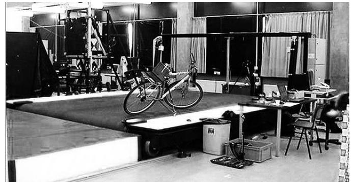
Figure 4. LARGE TREADMILL, 3X5 M, MAX SPEED 35 KM/H, COURTESY OF THE FACULTY OF HUMAN MOVEMENT SCIENCES, VU UNIVERSITY AMSTERDAM.
