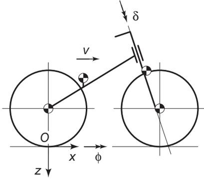
Figure 3. The bicycle model: four rigid bodies (rear wheel, rear frame, front handlebar assembly, front wheel) connected by three revolute joints (rear hub, steering axis, front hub), together with the coordinate system, and the degrees of freedom.
