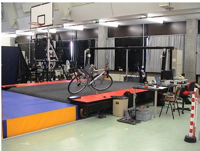
Figure 1. Large treadmill, courtesy of the faculty of Human Movement Sciences, Free University of Amsterdam, together with TUDelft instrumented bicycle.
