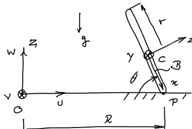
Figure 1.11: A disk rolling in a steady motion.
