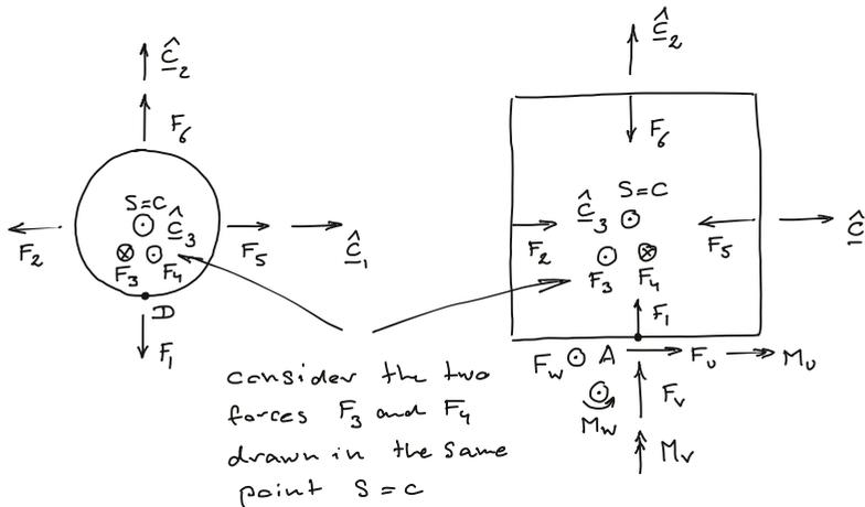
Figure G.4: Free-body diagrams for the accelerometer.
