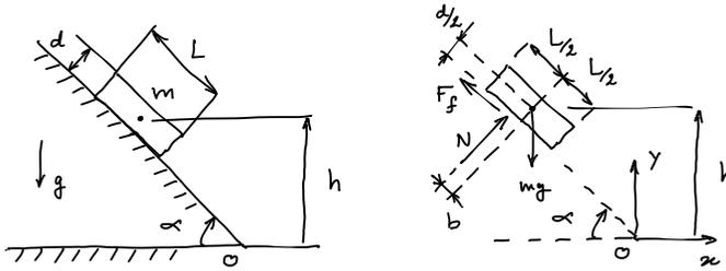
Figure 1.8: Sliding block and corresponding FBD.
