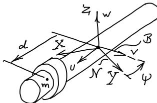
Figure 1.9: A rotating bar and sliding ring.
