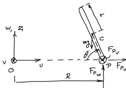
Figure G.1: Disk free-body diagram.
