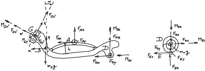
Figure G.5: FBDs of the scooter's footboard and rear wheel.
