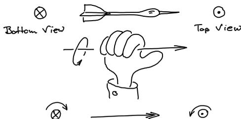
Figure 1.3: Notation for a vector that is perpendicular to the plane of drawing imagined as a dart (top); the right-hand rule to indicate positive direction of a rotation/moment about an axis (center and bottom).
