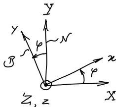
Figure G.7: Rotation of a coordinate triad about the  $Z$ -axis.
