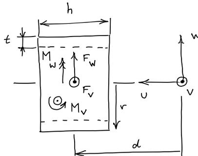
Figure 1.10: Free-body diagram of the ring.
