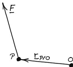
Figure 1.18: Illustration of a force and position vector of its point of application.
