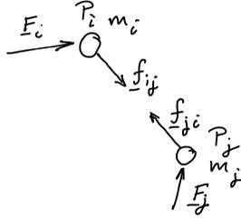
Figure 1.5: Two particles  $i$  and  $j$  with internal and external forces acting on them.
