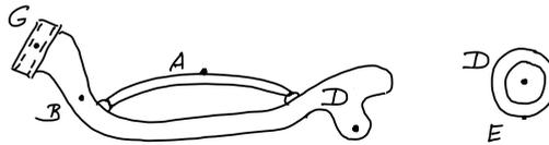
Figure 1.31: Scooter's footboard and rear wheel as free bodies.
