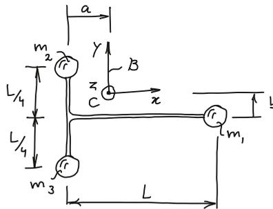
Figure 1.20: T-shaped rigid body consisting of three particles.
