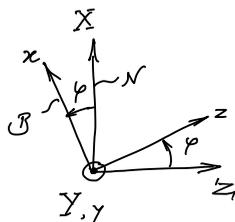
Figure G.8: Rotation of a coordinate triad about the  $Y$ -axis.
