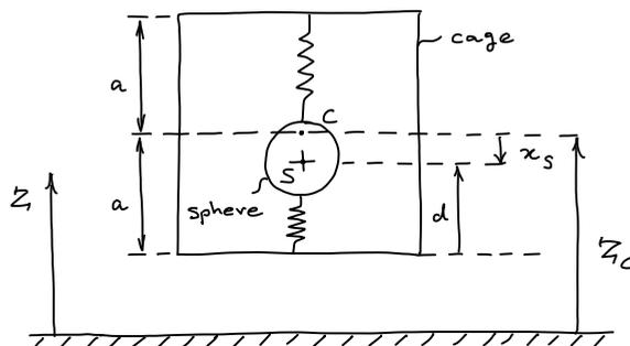
Figure 1.29: Kinematic diagram of simplified accelerometer in 1-D.
