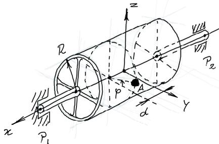
Figure 1.21: Unbalanced rotor.
