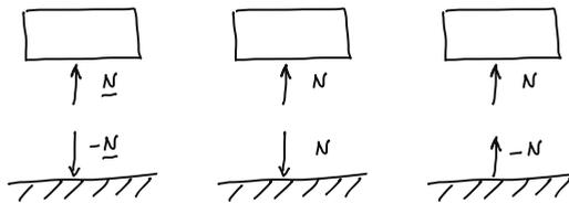
Figure 1.2: Equivalent drawings of force vectors, with vector (left) and scalar labels.
